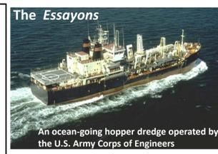
The hopper dredge *Essayons* utilizes a series of 12 doors located on the hull bottom to sequentially release each load of dredged material, resulting in a gradual release of dredged material from the vessel.
