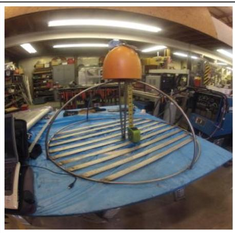
Deployable "deposition meter", designed for simplified deployment and retrieval similar to crab pots. A videocamera, was attached to the deposition meter mount, and recorded in-situ deposition and bottom-encounter physics resulting from dredged material placement. A staff gauge was attached to the center support element of the deposition meter. Three deposition meters were fabricated and deployed; each 13 inch high and 40 inch base dia. Photo, concept, and fabrication by CURTIS ROEGNER-NOAA.
