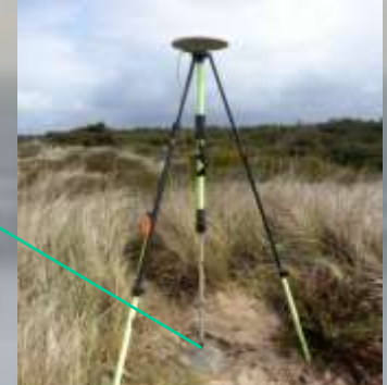
GPS Base Station
